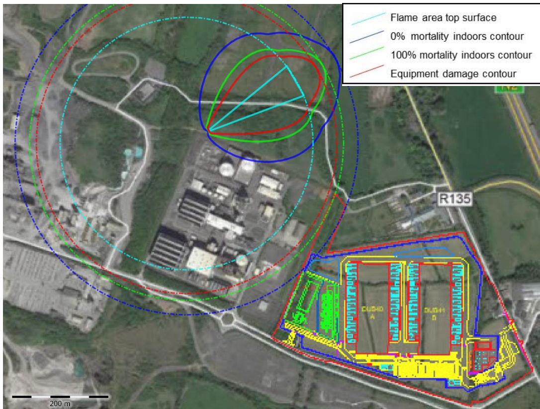
Figure 17 Natural Gas Jet Fire at GNI AGI: Indoor Mortality and Equipment Damage Contours
